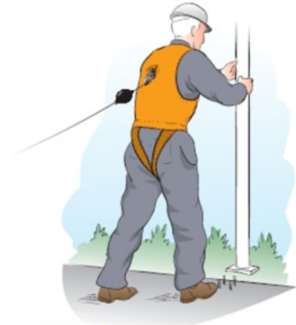
Personal fall protection equipment, full body harness sewn into the vest.
